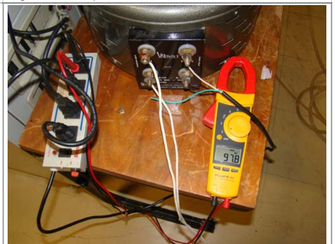
Figure 4. Initial setup of polarization: -15% of nominal voltage.
