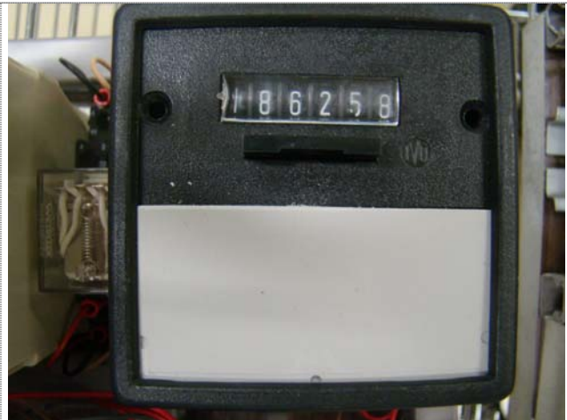
Figure 8. Counter of sample 60982 – 186,258 cycles (the time to each cycle was bigger than 30 seconds).
